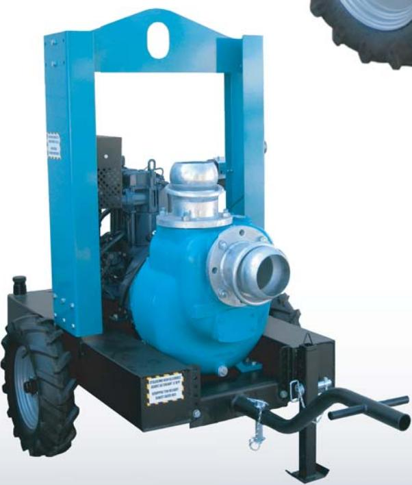
*Cast iron construction, internal nodular cast iron volute - plate, without screws, high hydraulic performance impeller with large solid passage, hard metal mechanical seal with innovative cooling system .*
